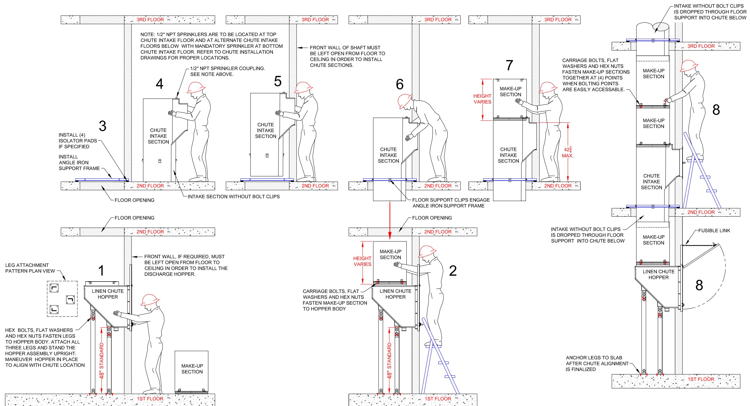
DISTRIBUTE CHUTE SECTIONS TO EACH FLOOR THAT IS TO BE INSTALLED
